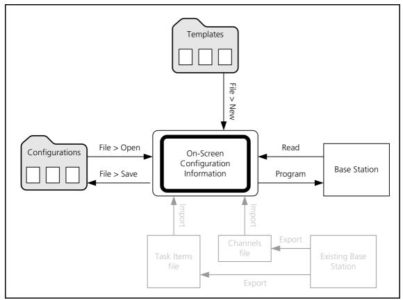
**Figure 1: Obtaining Configuration Information**
