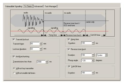
You can also set up a transmit lockout and enable anti-kerchunking.
