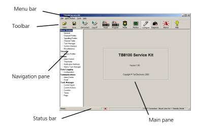
By default, the Monitor icon on the toolbar is selected and the navigation pane gives you options for monitoring. When you click an item in the navigation pane, the main pane displays the corresponding form.
