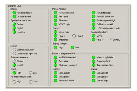
2. Look to see which LED is flashing red. A flashing LED means that the alarm is on. One problem can set off more than one alarm.
