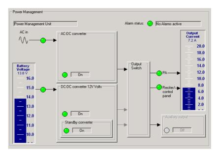
This form has a gauge displaying the battery voltage and another displaying the output current. Boxes represent different PMU submodules and LEDs indicate the status of power inputs and outputs. A box is disabled if the equivalent submodule is not installed.
