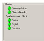
Power up failure The reciter has failed one or more of its initialisation self-tests and has gone into Download mode. The transmitter and receiver are disabled and any system interface outputs are deactivated.
