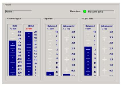
The first box in the form displays the internal name of the reciter.
