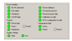
No PA detectedThe reciter cannot obtain a response from a PA over the using the control bus.<br/>The PA may still be operating but the system has lost the ability to monitor PA<br/>alarms, carry out diagnostics, change configuration, or detect PA fan failure.
