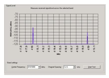
This test lets you see what signals are out there; it does not determine the receiver's sensitivity.
