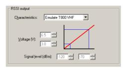
If the equipment is configured to operate with older Tait base stations, you can specify that the RSSI output behaves like the output from a Tait T800 VHF or UHF base station.
