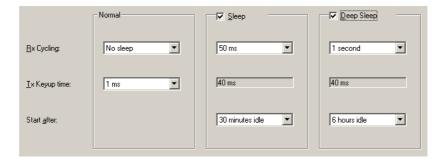
The base station begins in Normal mode. If the base station is idle (receives no <u>valid signal</u>) for a defined length of time, it switches to Sleep mode, which saves more power. If the base station is idle for a further defined length of time, it switches to Deep Sleep mode, saving even more power. When it receives a valid signal, it reverts to Normal mode.
