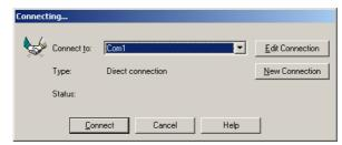
4. In the **Connect to** box, select Com1 or Com2, depending on the serial port you connected the cable to.
