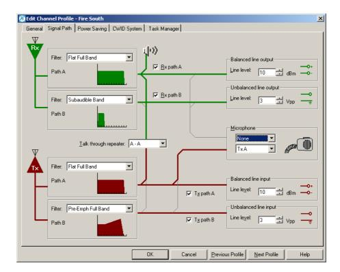
The left-hand side of the tab defines RF filter characteristics. Each panel has a drop-down list you can choose from, and a thumbnail graphic showing you the response characteristics of the filter you chose.
