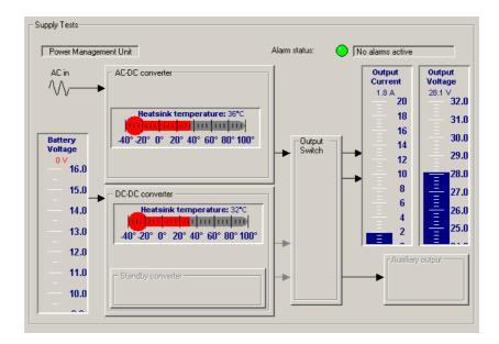
The form has a thermometer for each heatsink temperature sensor and an output voltage gauge. It also shows you all the monitoring information in Monitor > Monitoring > Power Management.
